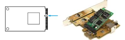
2. Once the mini PCIe card is fully inserted into the slot, push the card back against the adapter board. Fasten the mini PCIe card to the board with the small mounting screws provided. Make sure not to over-tighten the screws, or you may damage the mini PCIe card.
