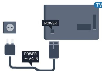
Although this TV has a very low standby power consumption, unplug the power cable to save energy if you do not use the TV for a long period of time.
