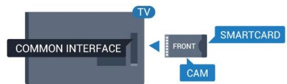
Use the Common Interface slot on the TV to insert the CAM card.
