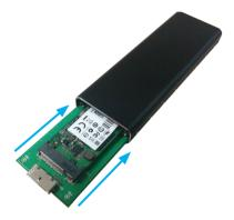
5. Using a Philips head screw driver (not included), replace the 2 drive tray screws on either side of the USB 3.0 Micro B port, on the front of the enclosure.
