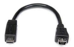
The UUSBMUSBMF6 Micro USB to Mini USB 2.0 Adapter Cable features a Micro USB male (B-type) connector and a Mini USB female connector, providing a cost-effective and convenient solution that lets you use a Mini USB cable to sync and charge Micro USB devices such as BlackBerry® or Android-based cell phones.
