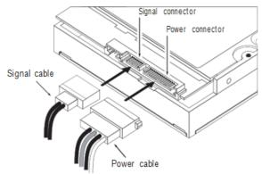
Each cable is keyed to ensure correct orientation. Seagate BarraCuda drives support latching SATA connectors.
