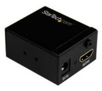
This HDMI signal booster lets you increase the signal strength of your HDMI video source so you can connect an HDMI display up to 115 ft. (35 m) away, using standard HDMI cables. You can place the booster inline between two HDMI cables, up to 82 ft. in length at the video input, and up to 33 ft. in length at the video output.
